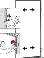
TIP: For doors without a threshold, a board can be used as a spacer in the frame opening to facilitate
